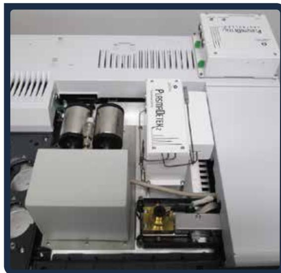
This figure shows an example of a simple sampling panel for the introduction and injection of a hazardous gas-liquid to GC. This is necessary for both accuracy and precision with these types of samples. The panel also allows for the safe venting of all hazardous samples to scrubber, with no dead legs, no dead volume, and no interaction of the sample with air. Applicable gas-liquids include: liquid chlorine, trichlorosilane, and tetrachlorosilane.
